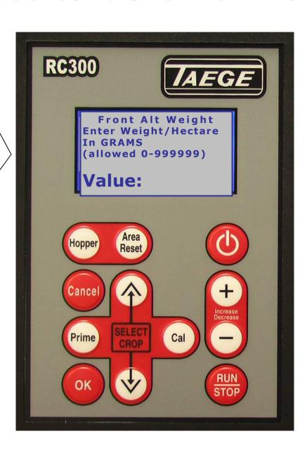
The Alternate Weight can be preset for all crop settings and on all hoppers. It can be more or less than the Target weight. Mainly used where variable ground conditions demand different seeding rates. This setting changes the seeding rate instantly whilst on the move by pressing the PRIME button, returns to the target weight when the PRIME button is pressed again. Seeding rates can also be changed on the move simply by
