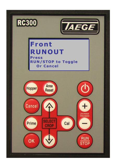
The Run to Empty function is used to assist the cleanout of the hopper between different crops
