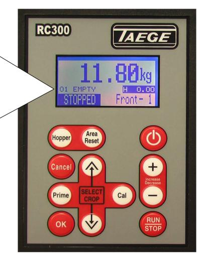
The **TOTALS MODE** screen enables the operator to record the last 5 reset areas for each crop setting. The controller can retain 5x25=125 area totals for each hopper
