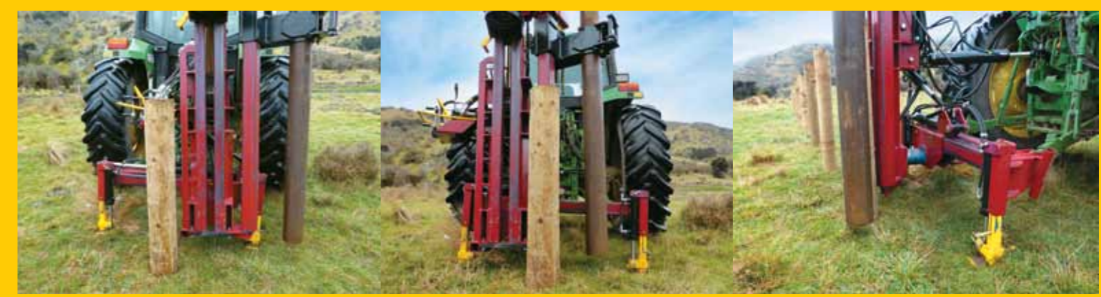
With a massive 600mm side shift, 170mm end shift and independent hydraulic legs on the Taege post driver, it gives plenty of movement to insure straight spiked holes and, in turn, straight posts
