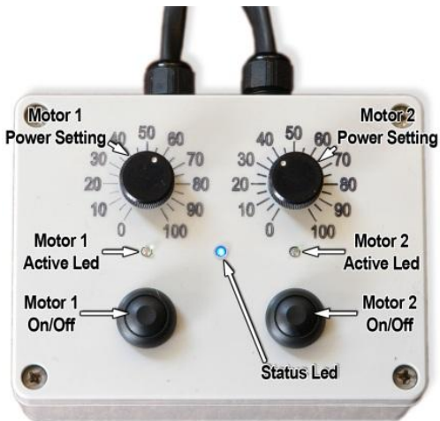
Figure 1: Control Layout and Indicator LEDs
