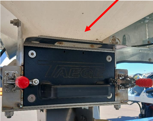
Inserted Metering Cassette with Over-Centre Clamps
