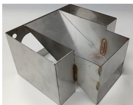
Hopper Emptying Chute
