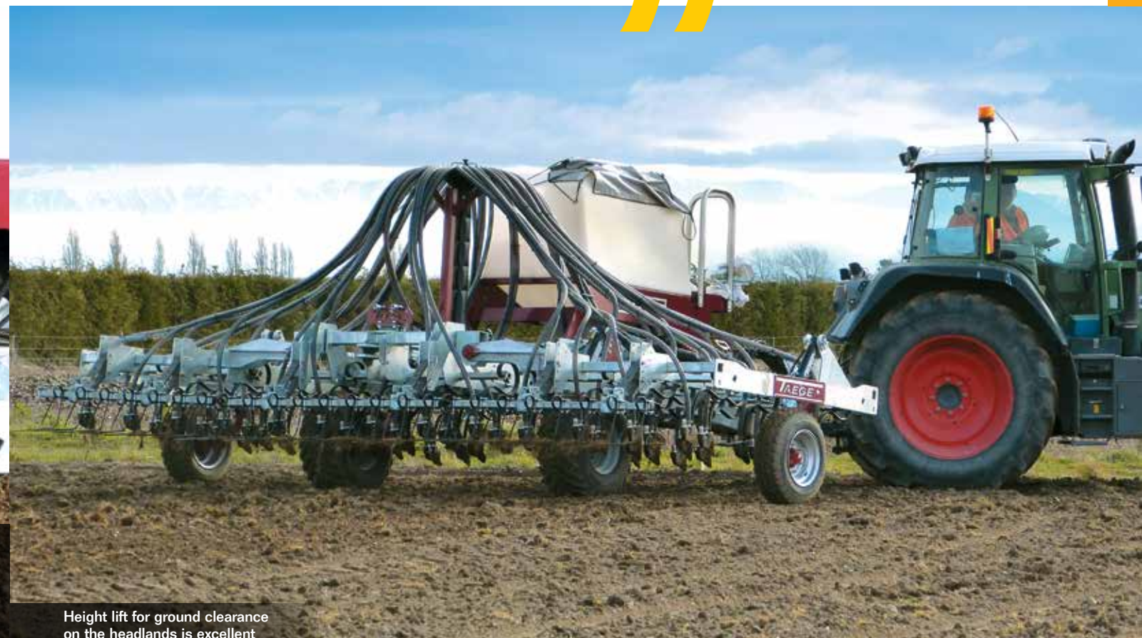
'S' shaped spring tine mount onto the box section that is rotating forward. This causes the tines to pull themselves into the ground with little downforce
