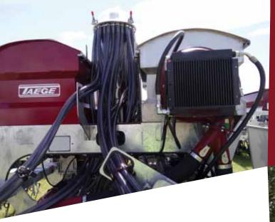
Tall distributor tower enables seed to run correctly on the top side of the hill.
