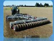
Taege hydraulic folding tyre rollers range from 3.6m to 6.0m. They can be configured to suit your requirements as far as folded and unfolded widths go. (Depending on tyre overlap and wheel offset)
