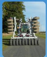
6.0m folds UNDER 3.1m allowing for towing on the road with over width panels.
