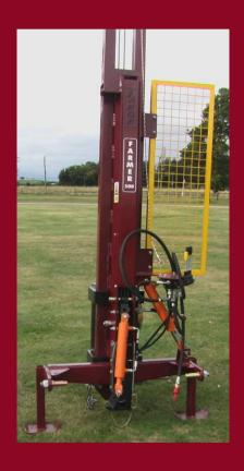
Farmer 500/700 showing the hydraulic top link and hydraulic angle shift.
